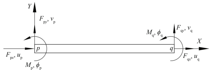
Fig. 5 Beam element with nodal displacements and forces
