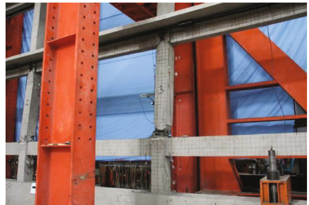
(b) Failure of column
