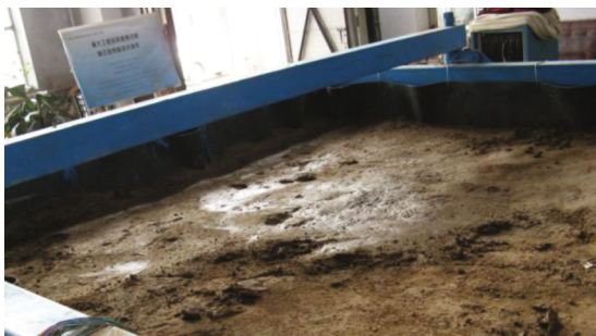
Fig. 5 Surface phenomena after the 0.4 g Taft-XZ loading case
