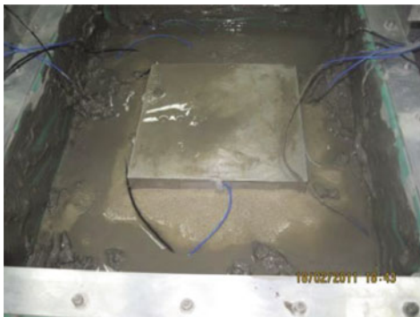
Fig. 5 Uplift of structure model in centrifuge test
