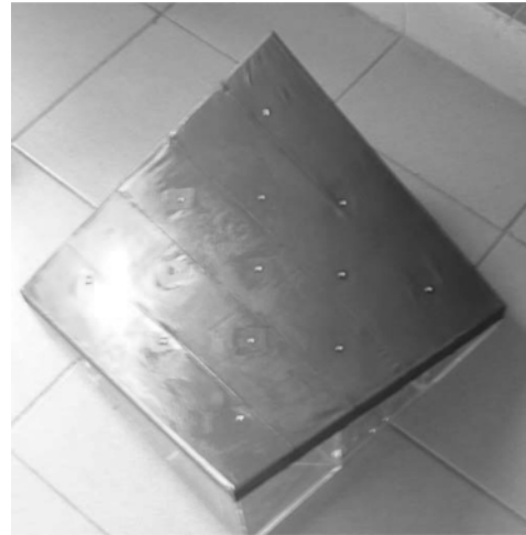
Fig. 14 Aero-elastic model for wind tunnel test
