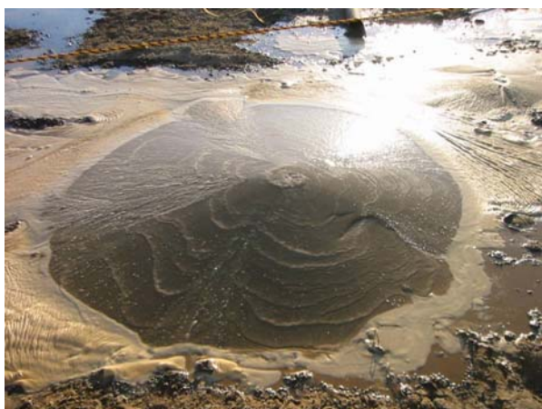
Fig. 6 Sand boil after 1 st test
