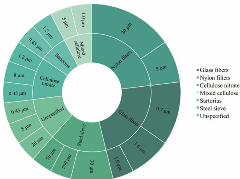
Fig.3 Commonly used filter membranes (inner ring) and pore sizes (outer ring) used in the reviewed paper for extracting microplastics.
