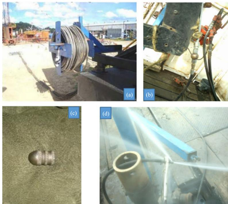
Fig.12 Injection tools for radial horizontal well. (a), high-pressure hose; (b), the connection between hose and coiled tubing; (c), injection bit; (d), pressure injection.
