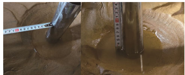
Fig.6 Scour morphology around a single pile.
