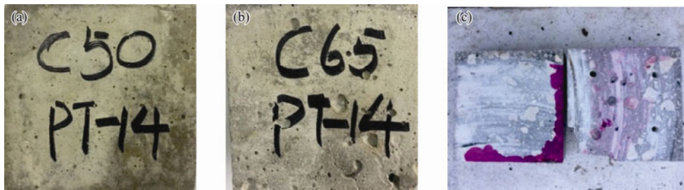
Fig.12 Surface state of CASC in the carbonation and drying-wetting cycles. (a), C50PT-14; (b), C65PT-14; (c), carbonation depth.
