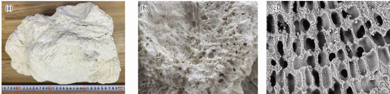
Fig.5 Porous structure of CASC. (a), coral-1; (b), coral-2; (c), coral-3.
