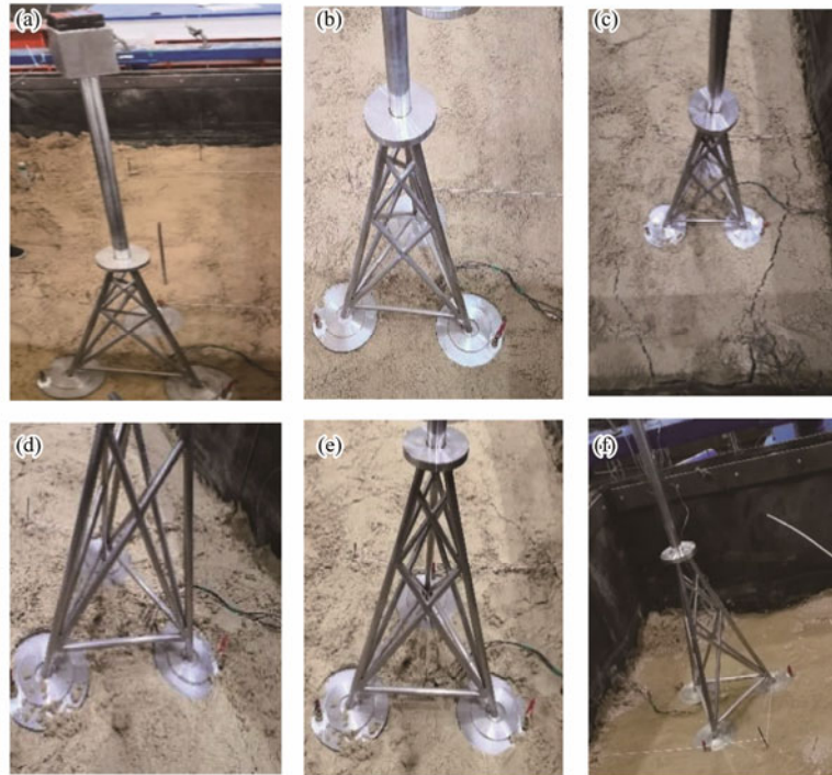
Fig.10 Process of model positioning. (a), model positioning; (b), sinking process; (c), cracks; (d), settlement; (e), settlement complete; (f), soil saturation.
