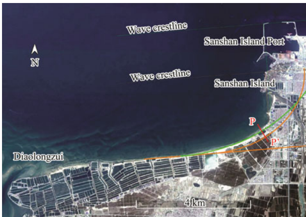
Fig.8 Simulation results for the Sanshan Island-Diaolongzui Shoreline. Green line is the simulation result as the corner point of Sanshan Island harbor is the updrift control point; Orange line is the simulation result as the rocky cape of Sanshan Island is the updrift control point.
