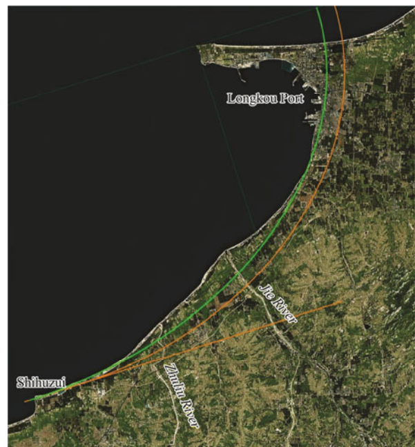
Fig.5 Simulation result for the Longkou Port-Shihuzui coast. Green line is the result of curve-fitting; Orange line is the location of the equilibrium coastline.
