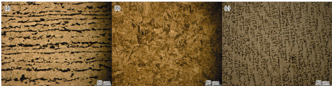
Fig.3 Microstructures of a) BM, b) HAZ, and c) WZ.
