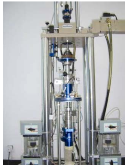
Fig.4 The triaxial cell of the soil static and dynamic universal triaxial and torsional shear apparatus.
