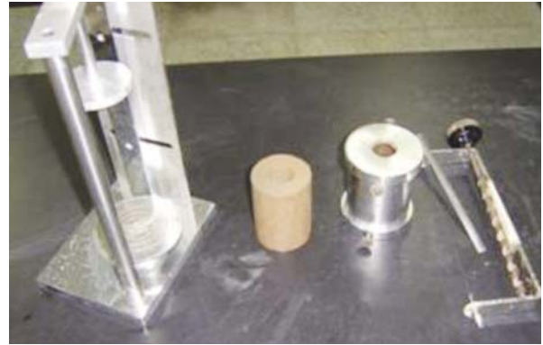
Fig.2 Tools for preparing samples and hollow-cylinder sample.
