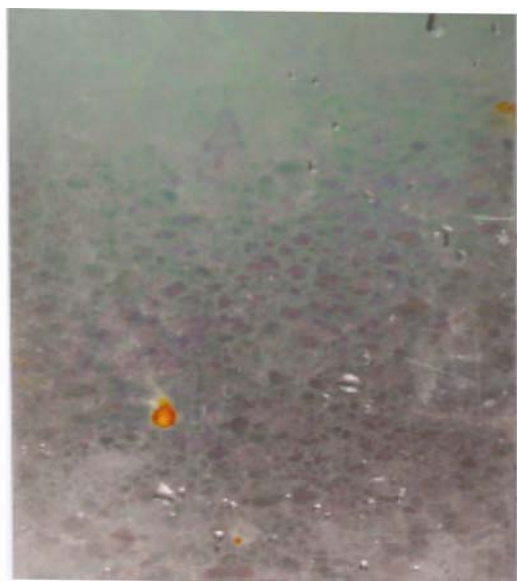
Fig.1 An optical micrograph of Ni-P deposit surface after standard salt spray test.
