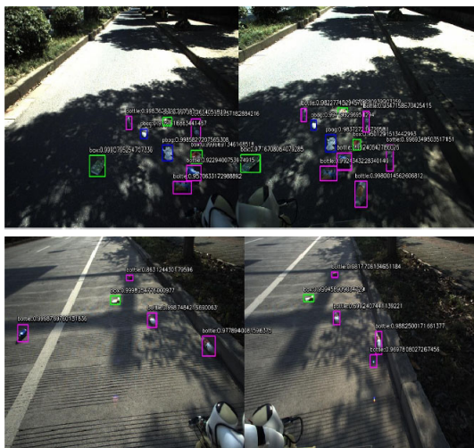
Fig.8 Actual detection results, where two images on the left and right represent the images collected by the left and right cameras
