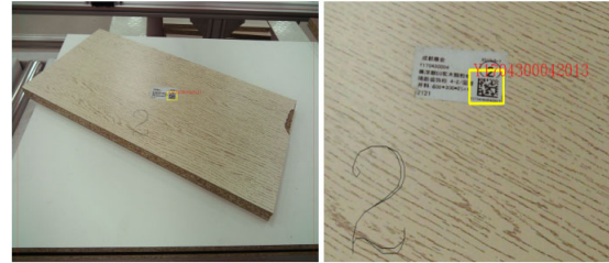
Fig.2 (a) QR code detection and (b) QR code recognition
