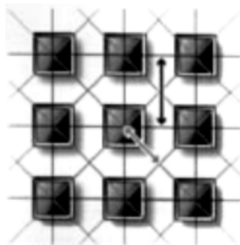
Fig.2 Structure of area array CCD pixels
