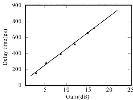
**Fig.6 The pulse delay under increasing  $G$**
