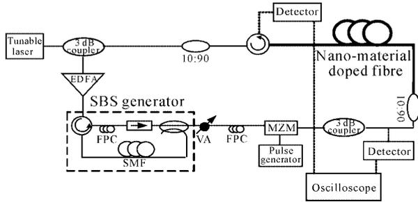
Fig.1 Experimental setup of SBS slow light
