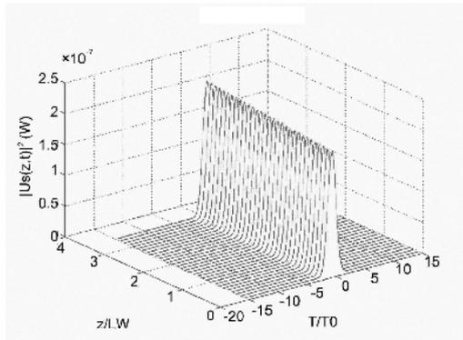
**Fig.4 The propagation of the Stokes wave**
