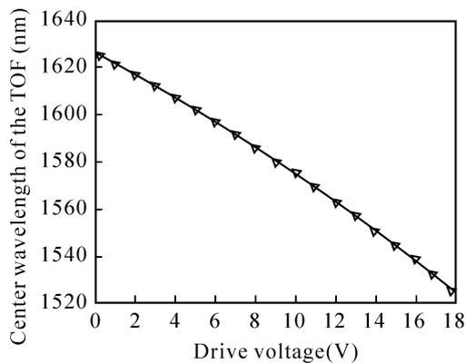
**Fig.3 Relationship between the transmission wavelength of the TOF and its drive voltage**
