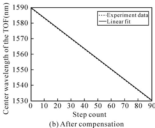
**Fig. 4 Transmission wavelength of the TOF**
