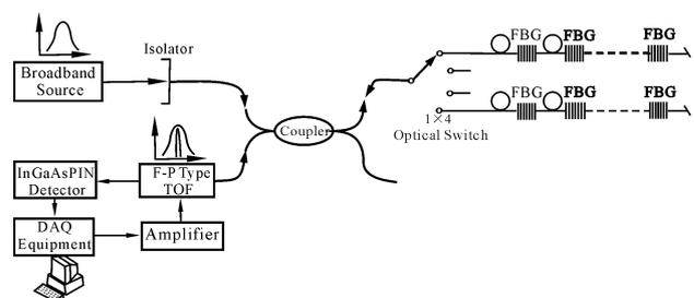
**Fig.1 The schematic diagram of the dynamic strain sensing system based on F-P type TOF**
