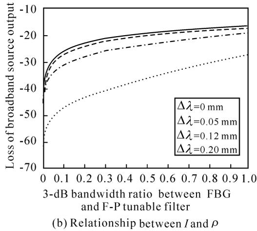
**Fig.2 The detected optical power as the function of  $\Delta\lambda$  (a) and  $\rho$  (b)**
