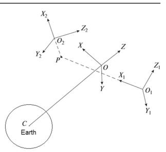
The indices i = 1 and i = 2 refer to body 1 (satellite) and body 2 (stabilizer), respectively. Consider the case when the hinge is located at the intersection point of the  $O_1x_1$  and the  $O_2x_2$  axes.
