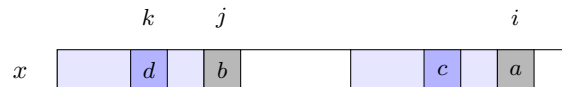
Fig. 15 kmp_x^1[i] = \{(k, j) \mid x[0..j-1] \text{ is a border at Hamming distance 1 of } x[0..i-1], x[k] \neq x[i-j+k] \text{ and } x[j] \neq x[i]\}
