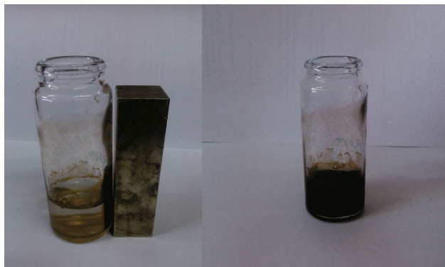
Fig. 8 Photographs of aqueous dispersions of MNPs modified with SDS in presence and absence of magnetic field
