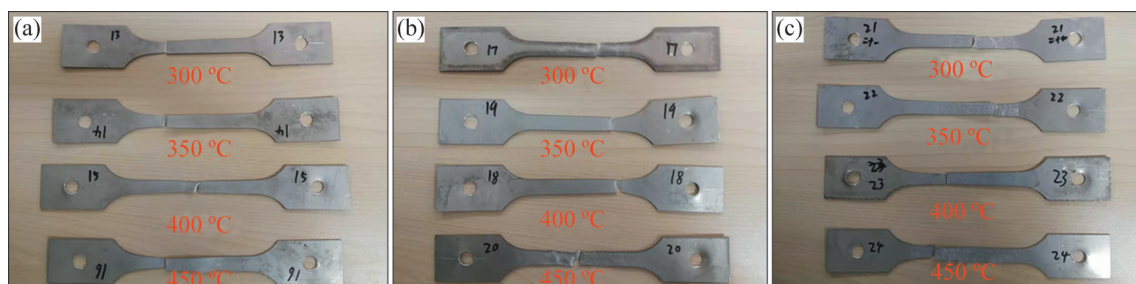
Figure 5 Broken test pieces when strain rate is 0.01\text{ s}^{-1} : (a) \epsilon_0=4\% ; (b) \epsilon_0=9\% ; (c) \epsilon_0=14\%
