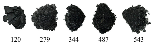
Figure 11 Failure patterns of coal samples under different loading rates during dynamic compression (unit: GPa/s)
