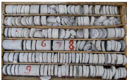
Figure 1 Typical core discing under high in-situ stress in Jinping deep tunnels
