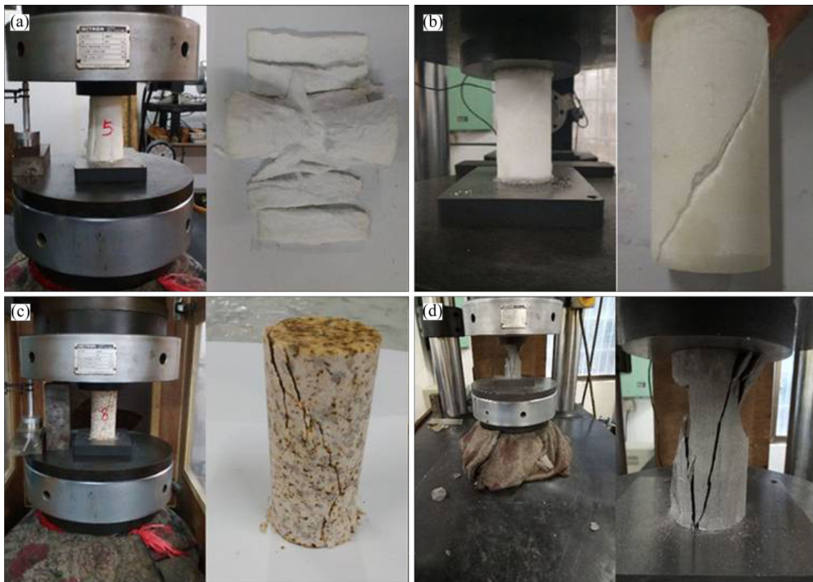
Figure 15 State of white marble, marble, yellow rust granite and black sandstone after failure: (a) White marble; (b) Marble; (c) Yellow rust granite; (d) Black sandstone
