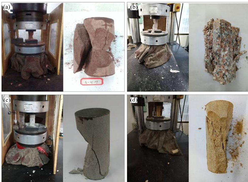
Figure 17 Situation of rock specimens after failure for medium rockburst proneness: (a) Red sandstone; (b) Red granite; (c) Green sandstone; (d) Yellow sandstone
