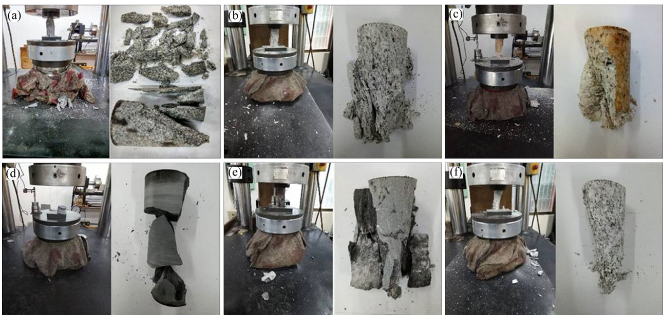
Figure 19 Situation of rock specimens after failure for high rockburst proneness: (a) Fine granite; (b) Yueyang granite; (c) Yellow granite; (d) Slate; (e) Limestone; (f) Qingshan granite
