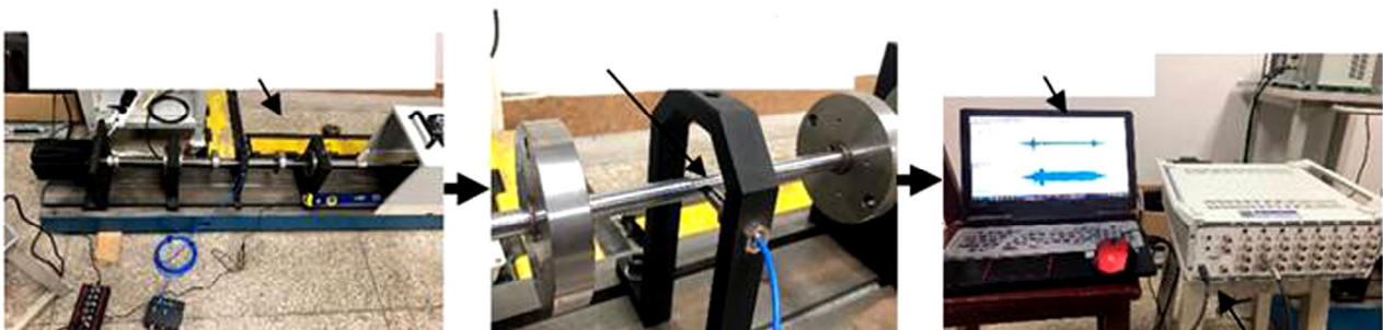
Figure 6 Multi-span rotor-bearing vibration test platform
