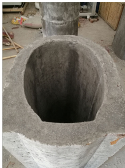
Figure 3 Tunnel lining model
