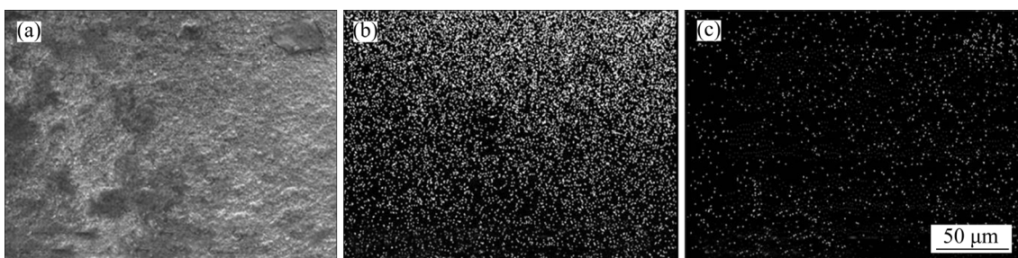
Figure 14 SEM image of zone 3 (a) and its elements map of tungsten (b) and carbon (c)
