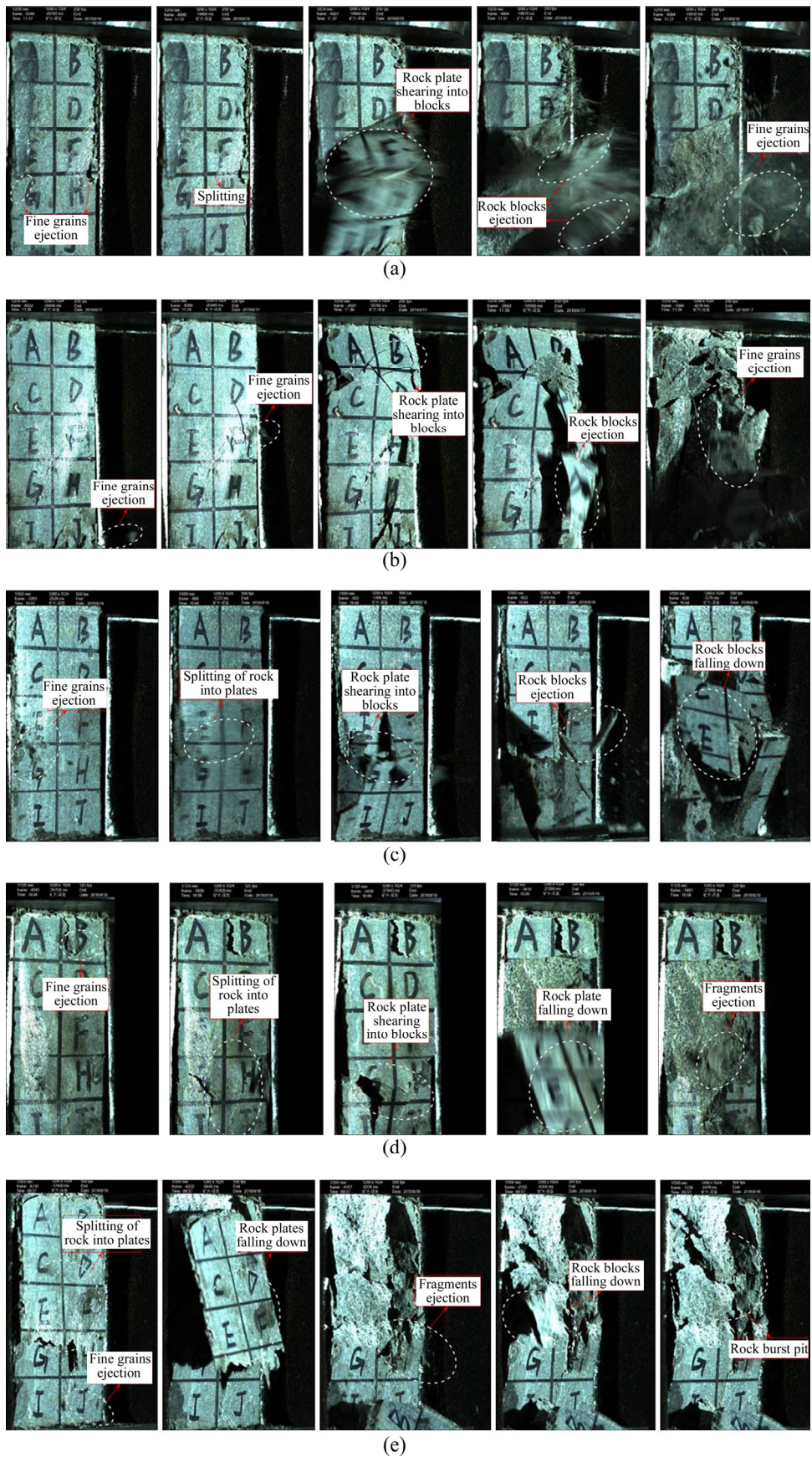
Figure 5 Strainburst process of rock specimens under different test plans: (a) G1-3; (b) G2-1; (c) G3-1; (d) G4-2; (e) G5-1
