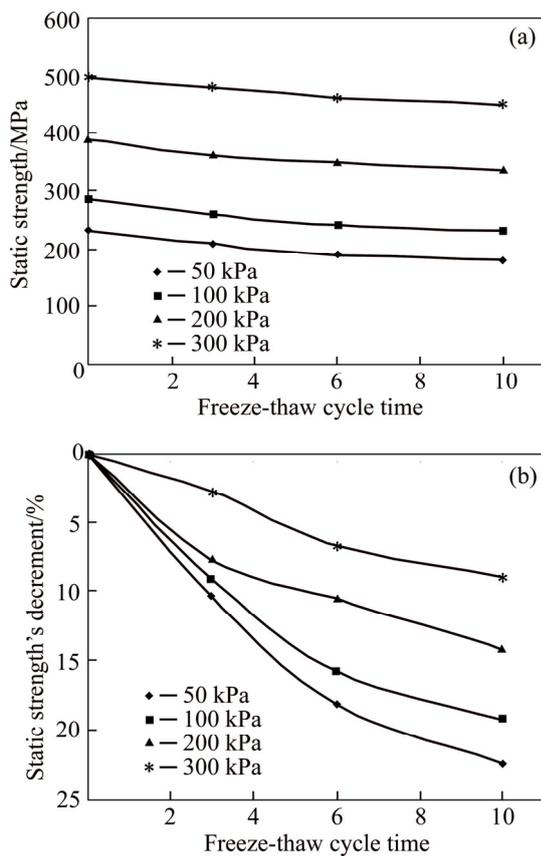
**Figure 4** Static strength’s decrement curves
