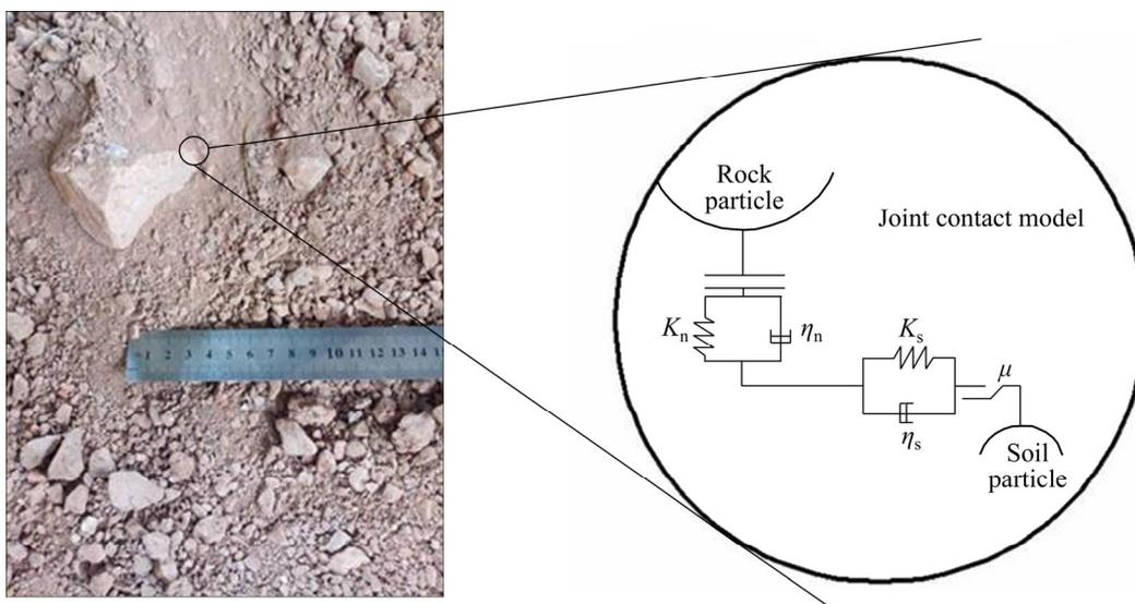
**Figure 8** Contact model between rock particles and soil particles
