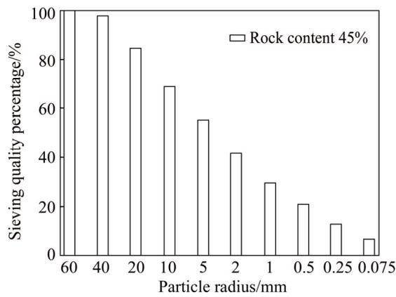
**Figure 1** Particle grading curve of sample with rock content 45%
