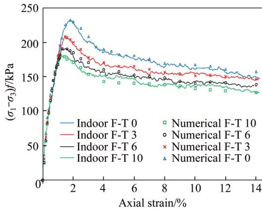
**Figure 10** Comparison between indoor curves and numerical curves
