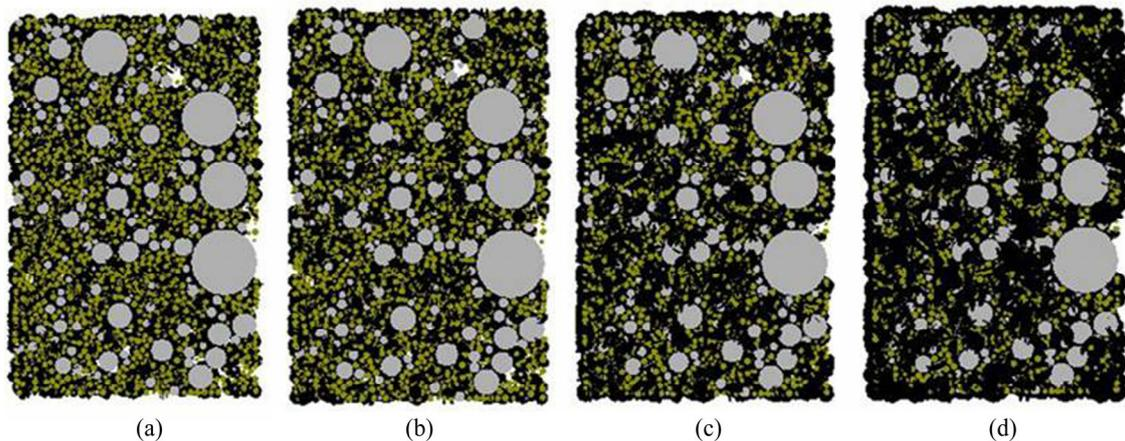
**Figure 11** Internal crack development after different freeze-thaw cycles: (a) 0; (b) 3; (c) 6; (d) 10
