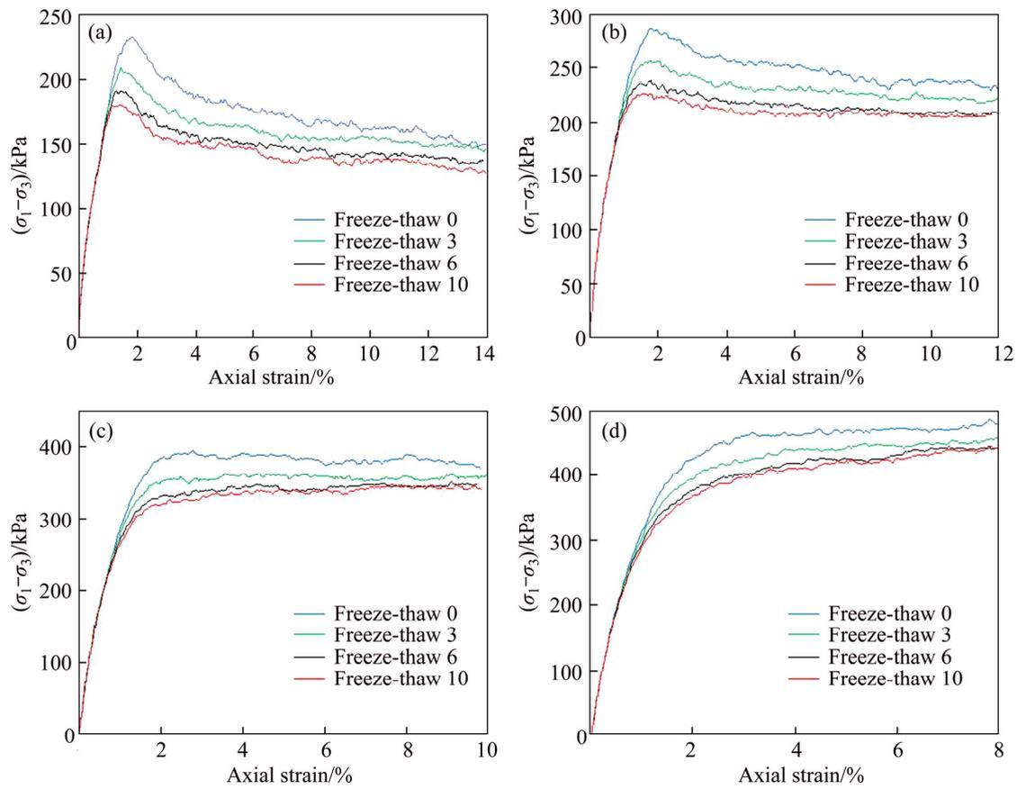
**Figure 3** Stress–strain curves after different freeze–thaw cycles under different confining pressure: (a) 50 kPa; (b) 100 kPa; (c) 200 kPa; (d) 300 kPa
