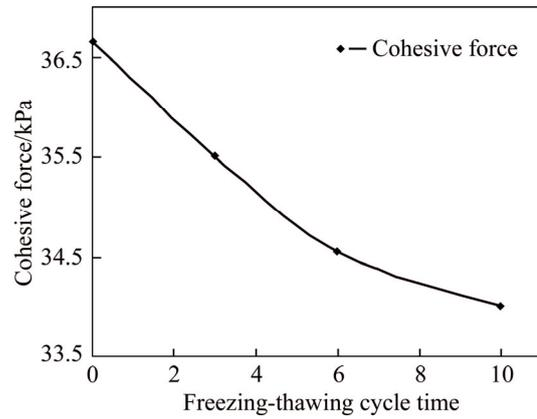
**Figure 6** Cohesive force's decrement curve
