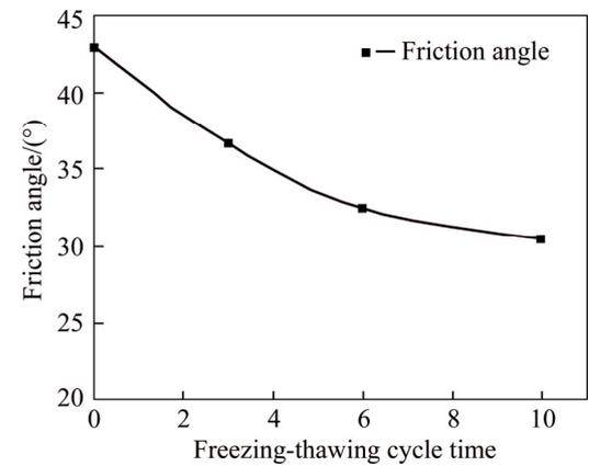
**Figure 7** Friction angle's decrement curve
