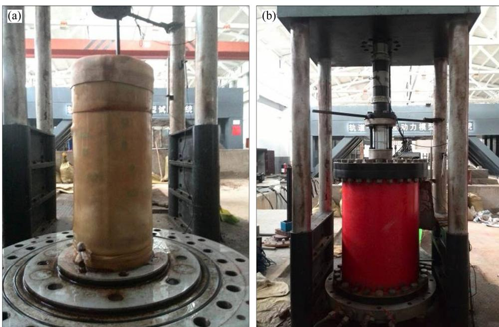
**Figure 2** Indoor triaxial freeze-thaw sample and equipment
