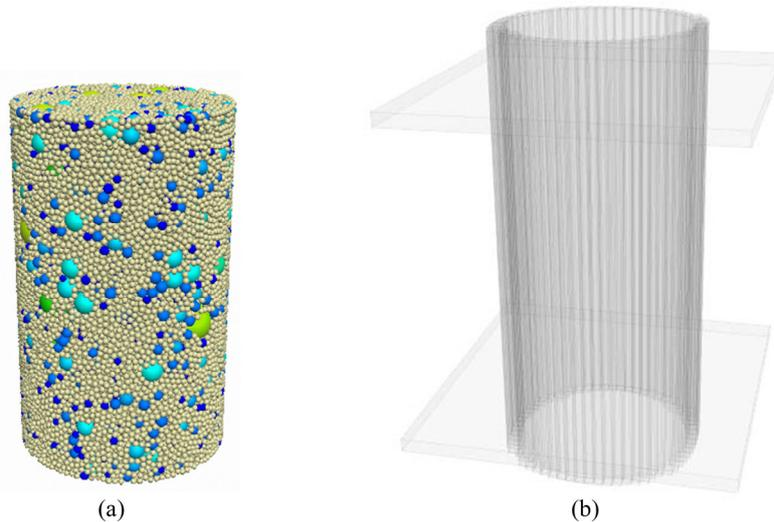
**Figure 9** PFC numerical simulation sample: (a) Triaxial numerical sample; (b) Triaxial restraint wall**Table 7** Parameters in PFC numerical simulation model
