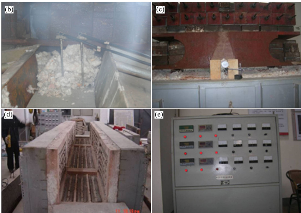
Figure 3 Specimen details and test setup: (a) Specimens details (mm); (b) Location of thermocouples; (c) Location of displacement transducers; (d) Layout of electric resistance furnace; (e) Layout of temperature control cabinet
