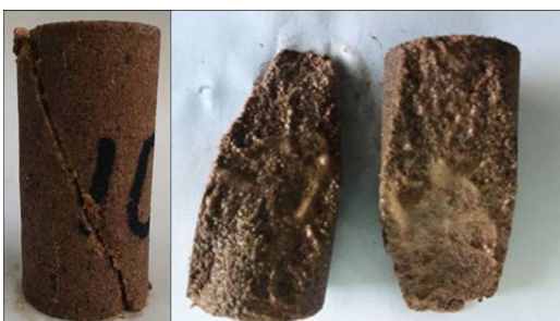
Figure 7 Typical pictures of failure pattern under confining pressure unloading condition
