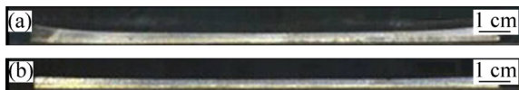
Fig. 10 Comparison of electroformed mold inserts without help of three validated methods (a) and with help of three validated methods (b)
