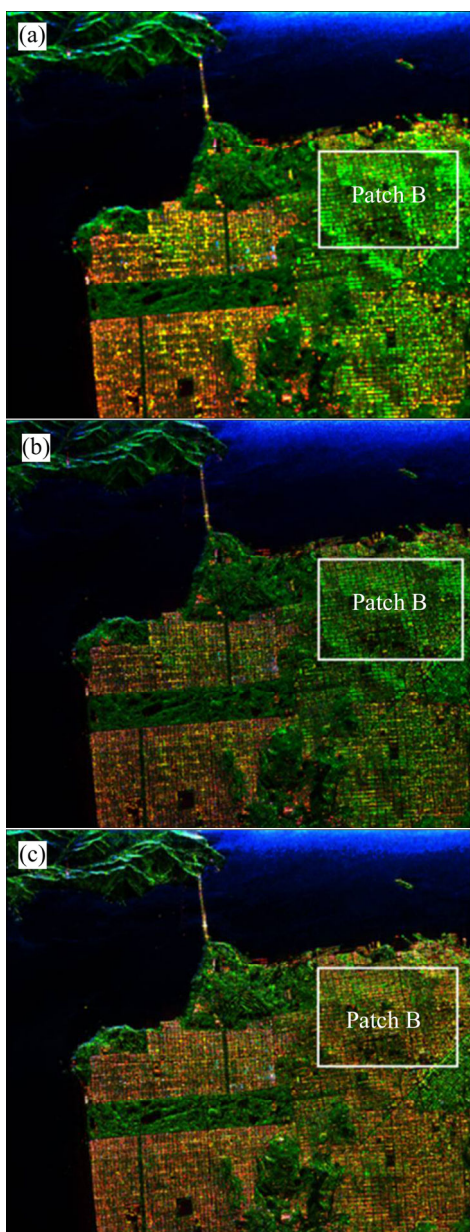
Fig. 4 Comparison of Freeman-Durden decomposition images that were filtered using: (a) 5×5 boxcar filter; (b) Lee’s SMB filter; (c) Improved SMB filter (The RGB images are color-coded: red for double-bounce scattering, blue for surface scattering, and green for volume scattering)
