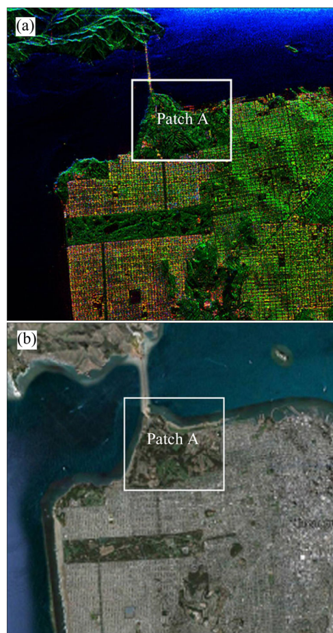
Fig. 2 Original Freeman-Durden decomposition image and corresponding optical image of San Francisco: (a) Original color-coded Freeman-Durden decomposition image (double-bounce scattering: red; volume scattering: green; surface scattering: blue); (b) Corresponding optical image from Google Earth
