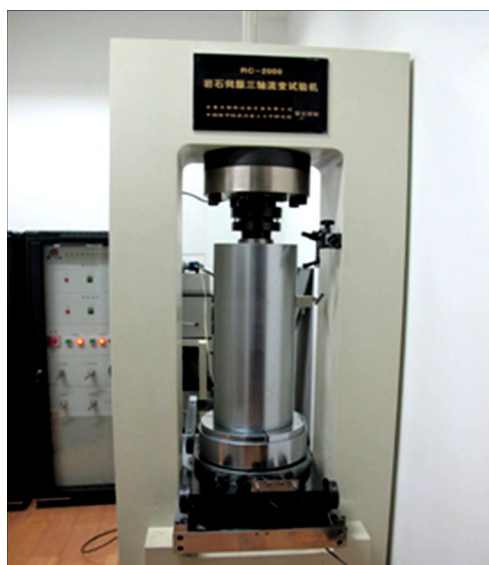
Fig. 1 TLW-2000 triaxial rheological testing machine with a high pressure confinement
