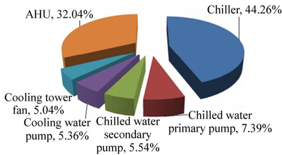
Fig. 3 Energy consumption structure of equipment
