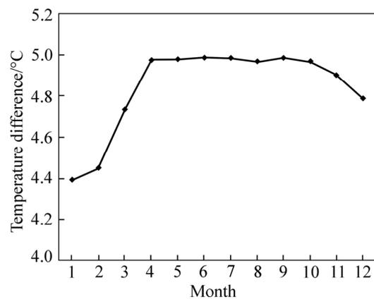
**Fig. 10** Monthly average cooling water supply and return temperature difference
