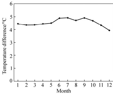
**Fig. 8** Monthly average temperature difference between the supply and return chilled water
