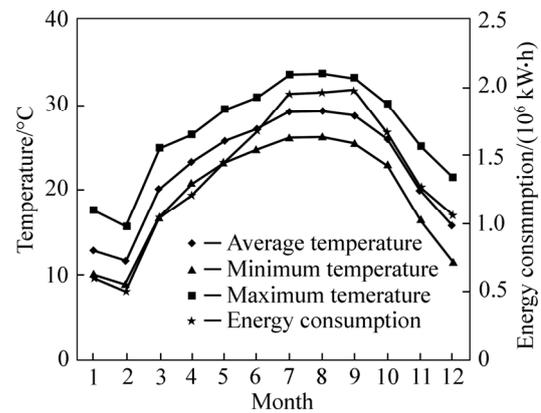
Fig. 4 Monthly average energy consumption of air-conditioning system and monthly outdoor temperature
