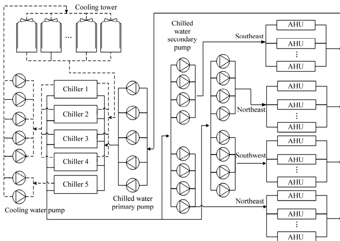
Fig. 2 Schematic of central air-conditioning plant
