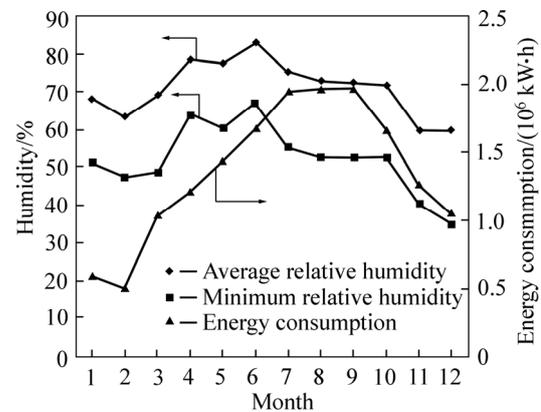
Fig. 5 Monthly average energy consumption of air-conditioning system and outdoor relative humidity
