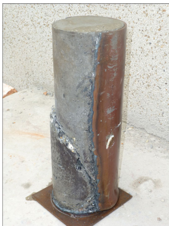
Fig. 2 Shear failure plane in concrete core
