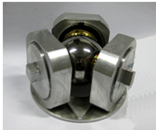
Fig. 9 Prototype of 2-DOF spherical ultrasonic motor
