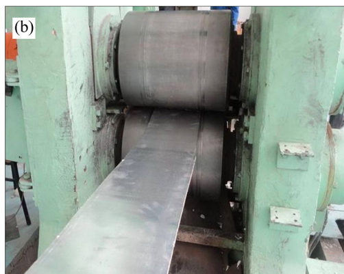
Fig. 1 Schematic diagram (a) and experiment photograph (b) of electromagnetic and ultrasonic cast rolling
