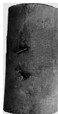
Fig. 2 Typical rock-like specimens prepared for laboratory test
