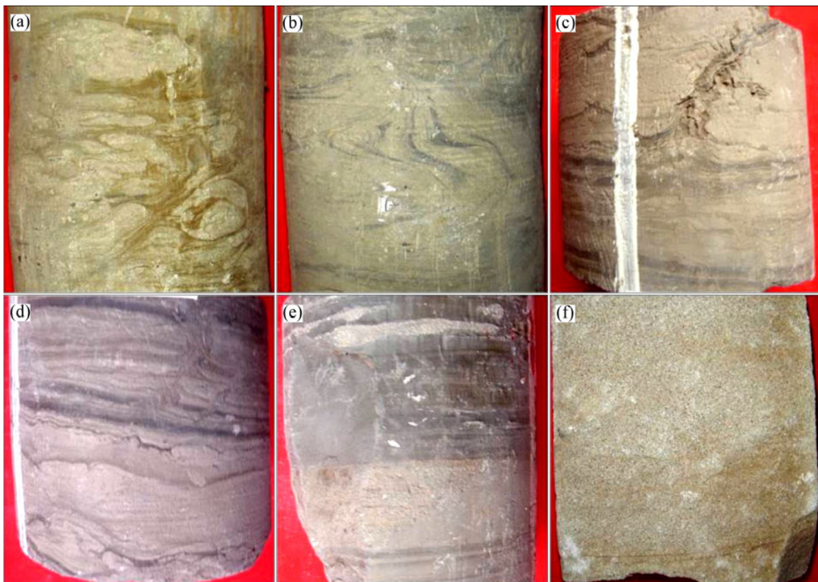
Fig. 2 Lithology and tectonic characteristics of sediment gravity flows in Gangzhong area: (a) Slump deformation structure, well z11-70, 2673.53 m, Es2; (b) Deformation structure, well z11-70, 2633.14 m, Es2; (c) Water escape structure, well gs56, 3190.31 m, Es2; (d) Slump deformation structure, well z11-70, 2673.53 m, Es2; (e) Sharp contact between well gs56, 3194.6 m, Es2; (f) Light gray medium sand, well z11-70, 2667.79 m, Es2
