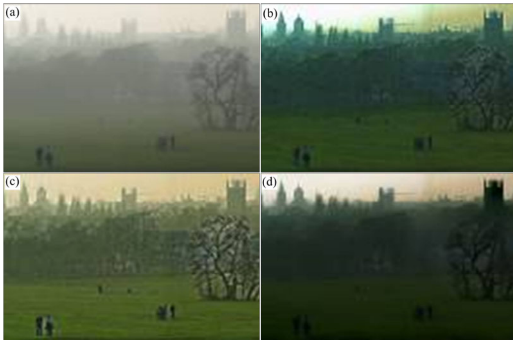
Fig. 5 Defogging effect comparison for real scene images (1): (a) Haze image; (b) TAN's result; (c) TAREL's result; (d) HE's result
