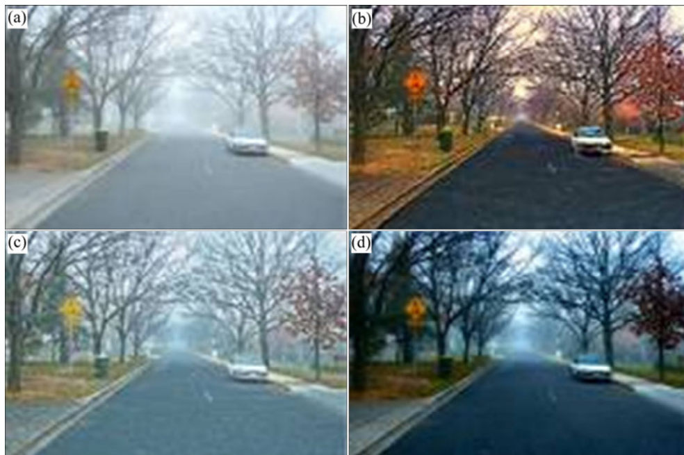
Fig. 7 Defogging effect comparison for real scene images (3): (a) Haze image; (b) TAN's result; (c) TAREL's result; (d) HE's result
