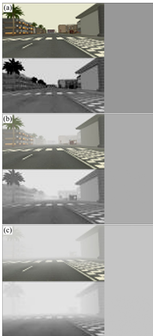
Fig. 4 Input (top), dark channel (bottom) and estimated fog veil images with different fog density: (a) No-fog; (b) Haze; (c) Dense fog
