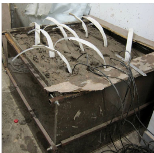
Fig. 4 Photo of test cell before reinforcement
