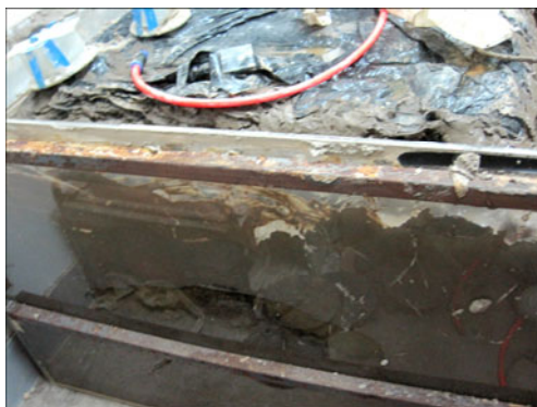
Fig. 9 Crack between test soil and cell wall due to lateral contraction
