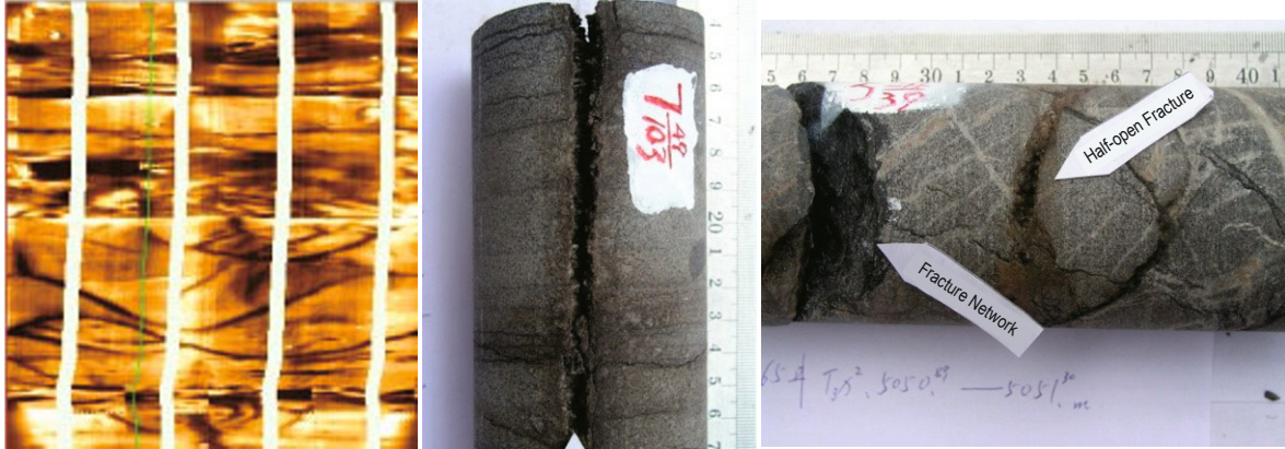
Fig.4 Formation fracture imager photo and core photos from Well CX560.
