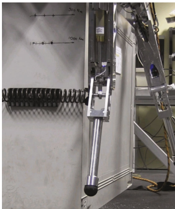
Fig. 13 Experimental setup for passivity tests. The rotational stiffness K_{L2} is obtained by positioning a linear spring at a certain distance from the HAA axis.
