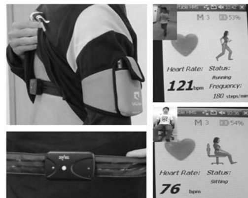
Fig. 2 uCare device worn on the chest and up arm (left). The sensor node has dimension of 56 \times 32 \times 16 mm and weight of 25 g (bottom left). The smart phone screens (right) show two scenarios of sitting and running, when the heart rate are 76 and 121 bpm, respectively. The running speed is 180 steps per minute.
