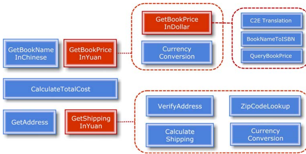
Fig. 2 Component WSs of a 3-level hierarchical online shopping scenario in which the service GetBookPriceInYuan and GetShippingCostInYuan are subprocesses. GetBookPriceInDollar in subprocess GetBookPriceInYuan is also a subprocess composed of WSs
