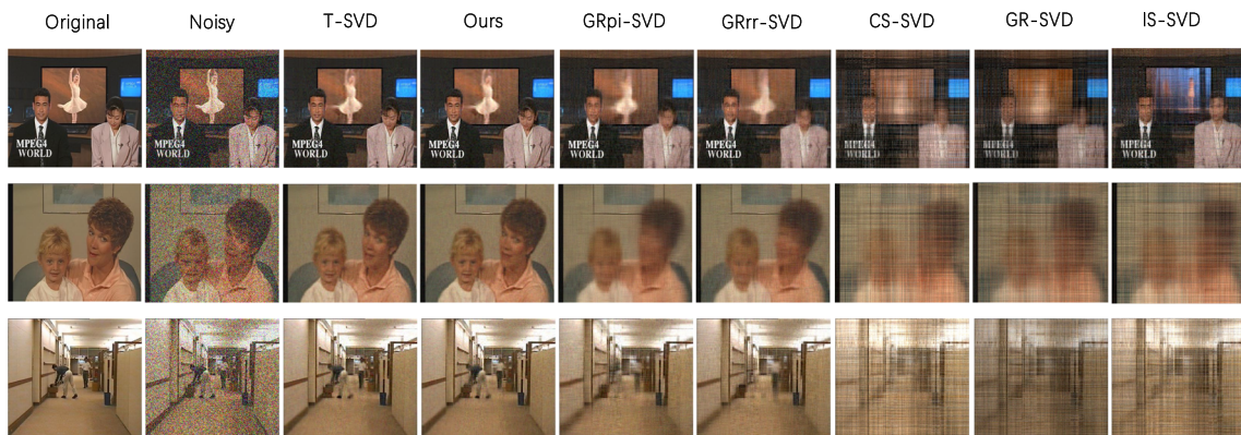
Fig. 3 Examples of video denoising, including original data, noisy data and recovered data. Our method achieves accurate approximations comparable to T-SVD, while in a more time-efficient fashion
