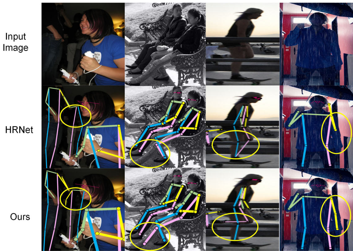
Fig. 9 Comparison of our method with HRNet method for pose estimation under adverse lighting conditions
